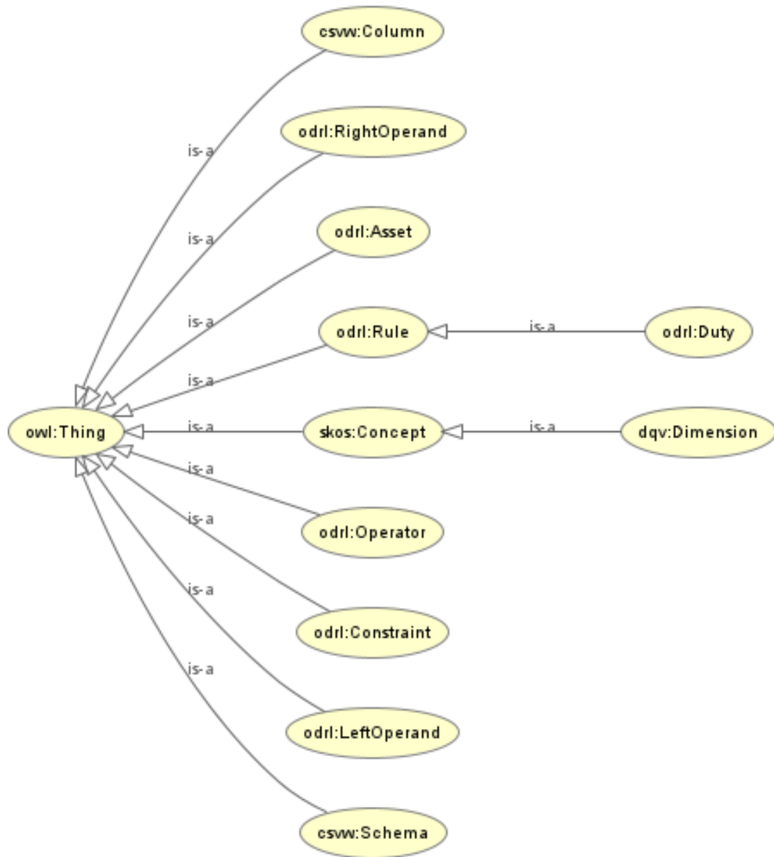
Figure 5.10: Class hierarchy of Dataset Schema Module through the OWLViz plugin in Protégé; prefixes denote the reference ontology
