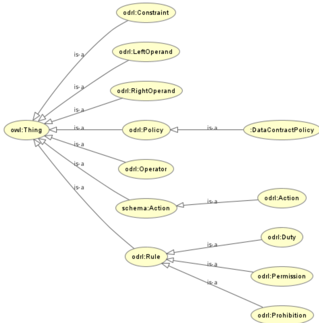
Figure 5.8: Class hierarchy of Data Contract Module through the OWLViz plugin in Protégé; prefixes denote the reference ontology
